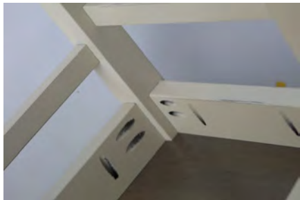
Mortise & tenon and Pocket screw construction
